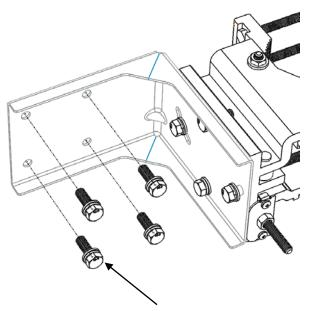
Attach 4 – 15mm M8 Bolts with flat and split lock washers to your MetroLing unit
