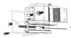
Center the vertical adjustment slide on the bracket
